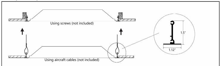
4. Place the kit in the ceiling opening and secure it with the screws.
